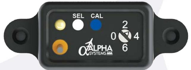
Cover the photo diode on the AOA DISPLAY with your thumb and wait 5 seconds.
