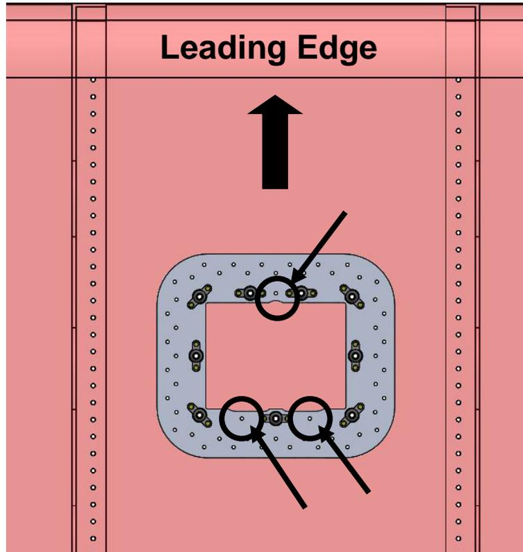
Drill out these 3 holes for reference and orientation for both the Doubler and Probe Mounting Template location.
