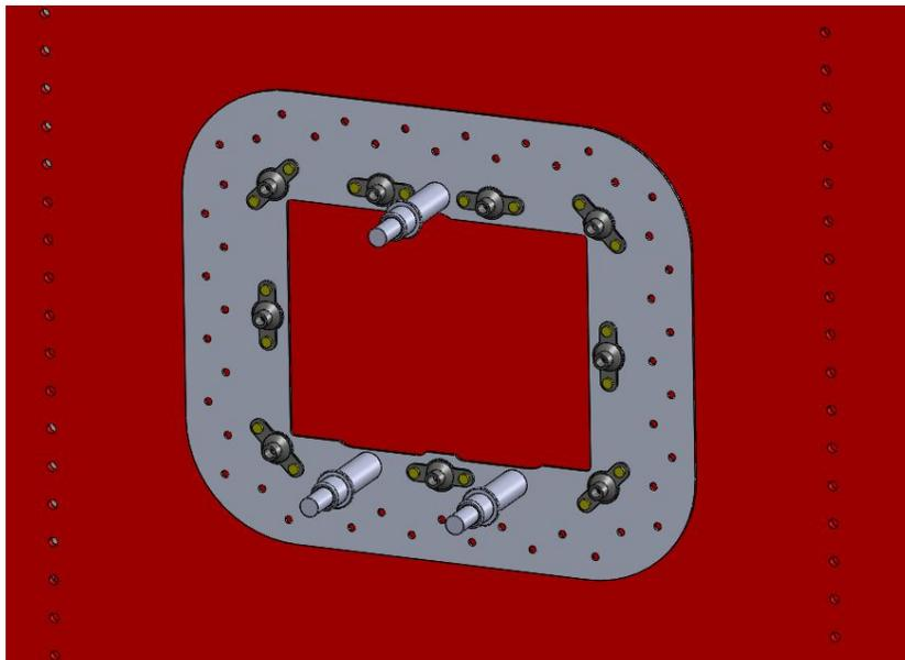
**STEP 3:** Remove doubler, debur drilled holes, and Cleco the AOA Probe Mounting Template (AOA-4203) using the 3 reference holes. Scribe/mark around the edge of the AOA mounting Template.
