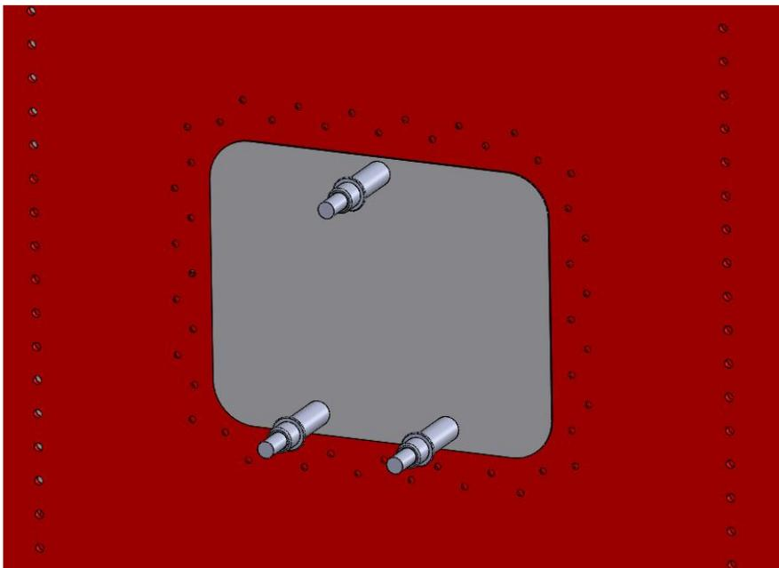
**Step 4:** Remove Template, discard, remove material inside scribe line, and make clearance so that the AOA probe mounting plate can be flush mounted when complete.
