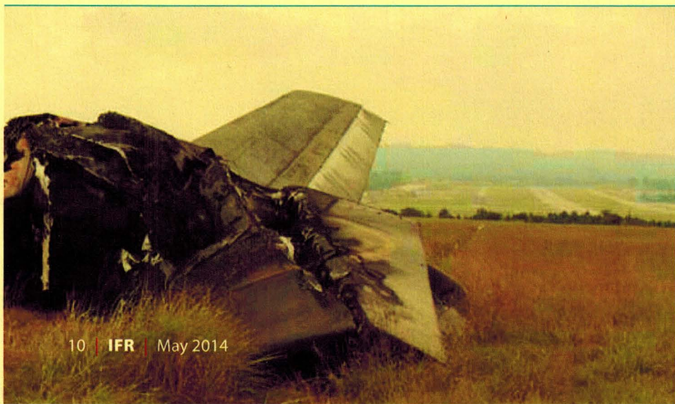
LEFT: Indications are that UPS 1354 chased the FMC glidepath below MDA, crashing just short of the runway.
