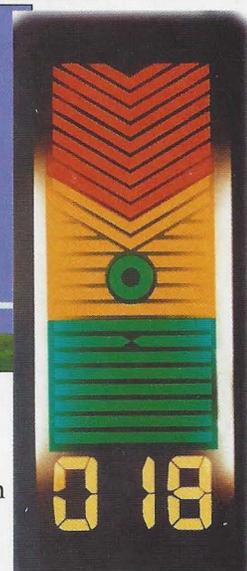
panel-mounted version. It's simple—aim for the blue LED when landing. The more LEDs that are on, the more lift you have.
