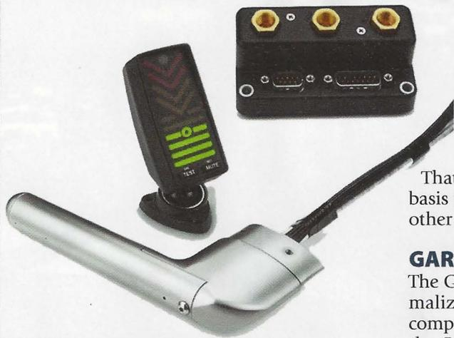
*Garmin's normalized AoA system, upper left, uses a pitot tube, an air data computer and a glareshield-mounted indexer, top picture. It's approved for certified aircraft independent of existing avionics. Alpha Systems, grouped upper right, has a seemingly endless variety of AoA displays options.*
