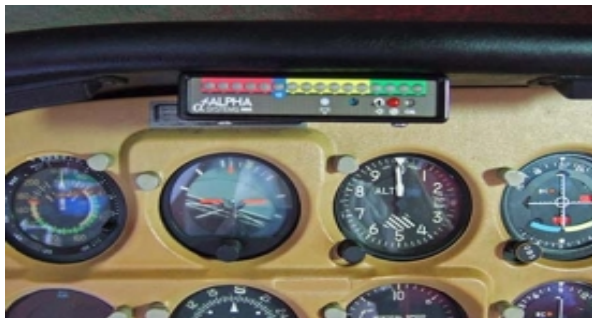
Angle of attack indicators could soon make their way to the owner-flown segment. Shown here, an AoA indicator in a Cessna 177 Cardinal. (Photo: Alpha Systems )
