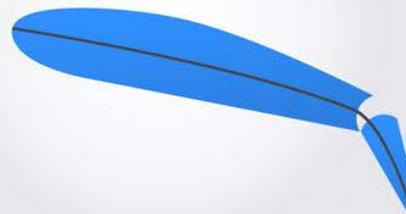
This all happens because extending flaps *increases the camber*, or curvature, of your wing. When your wing has a higher camber, it also has a higher *lift coefficient*, meaning it can produce more lift at a given angle-of-attack.
