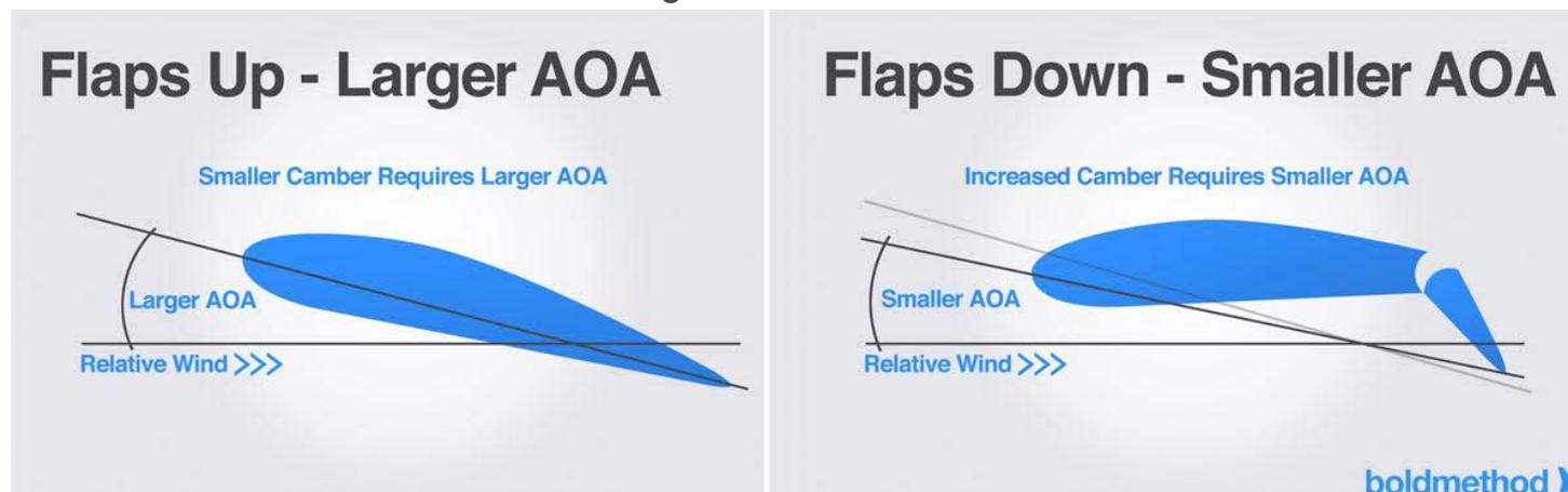
And because you can fly at a lower angle-of-attack with flaps extended, your stall speed will be lower as well.
