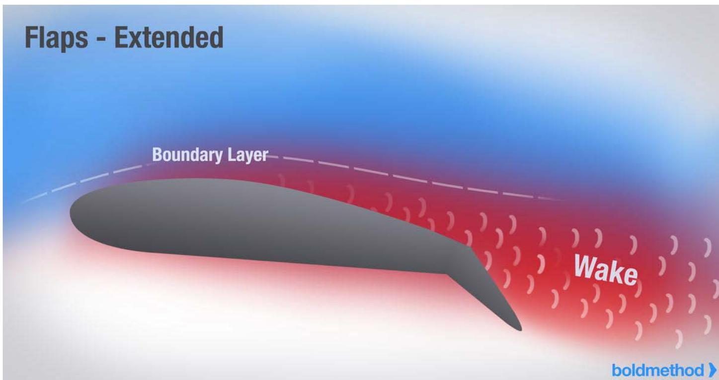
This is true for both large and small planes. Even for a Cessna 172S, 10 degrees of flaps are recommended for takeoff.
