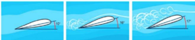
Figure 1: Wing Flow Separation at Stall
