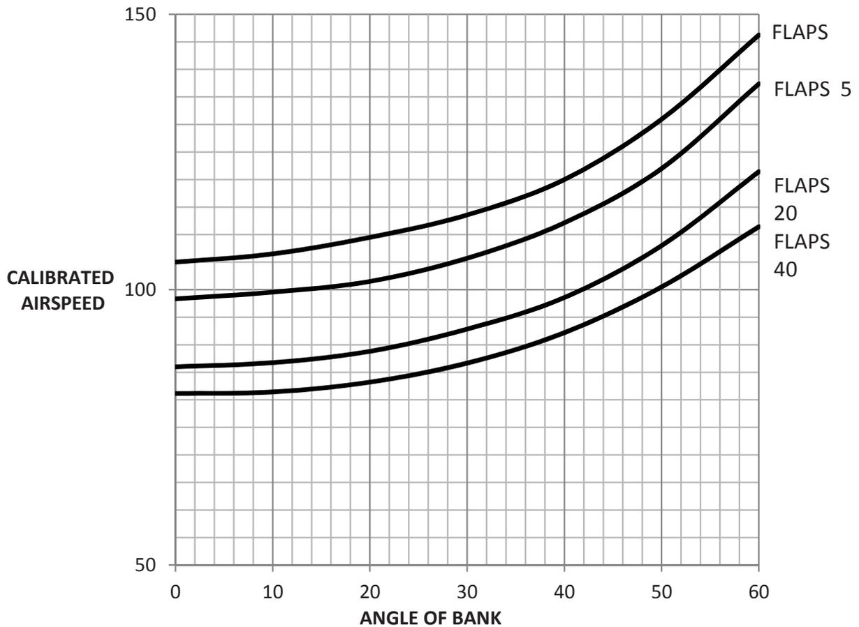
Figure 4: Stall Speed vs Angle of Bank MU-2B-60
