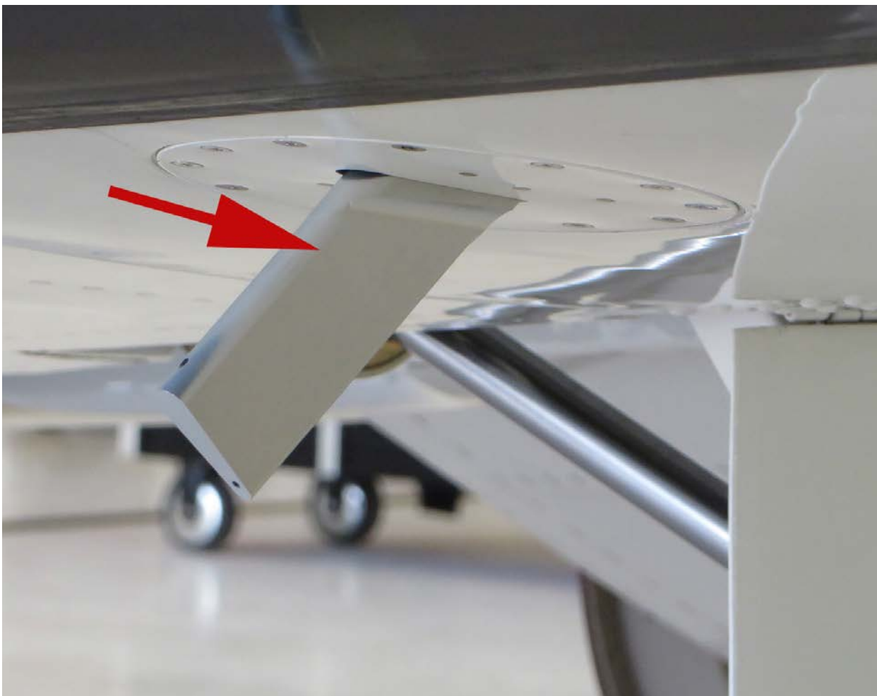
AoA heated probe mounted to LH wing inspection panel outboard of MLG door.
