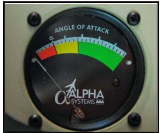
Needle high? Push it down, or relax a bit of back pressure. Needle low? Pull it up.
