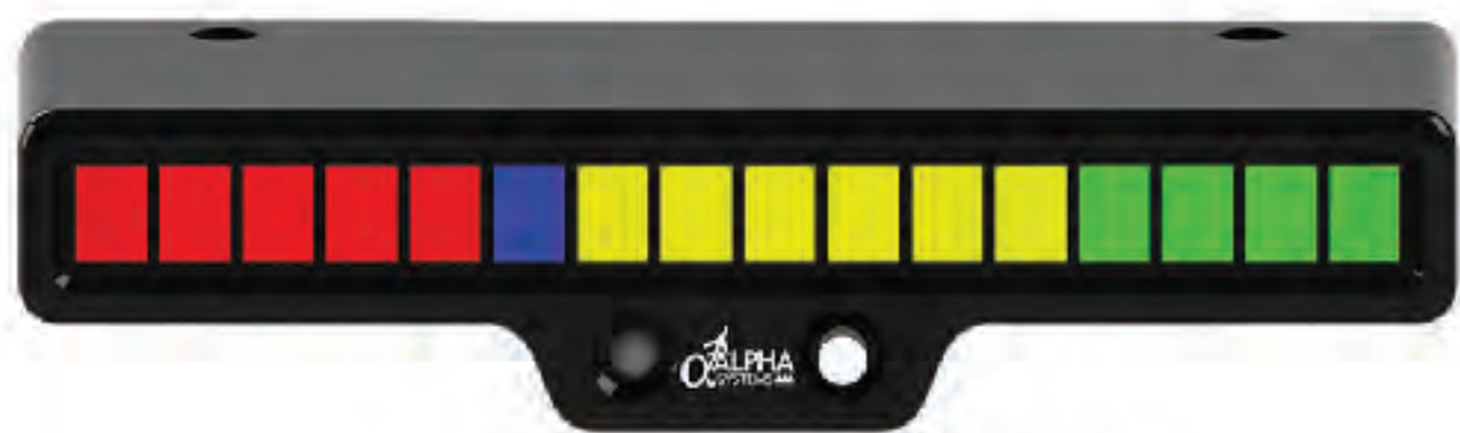
Merlin Display display shown with all segments illuminated
