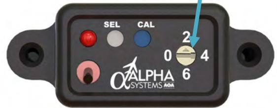
**Note:** When at the maximum volume level, the unit will announce “Maximum Volume Reached.” When at the minimum volume level, the unit will announce “Minimum Volume Reached.”
