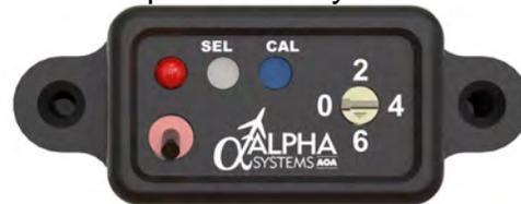
**Calibration Mode Rotary Switch:** Is an 8 position rotary switch that uses the **WIDE PART OF THE SLOT** to indicate the switch position, **NOT THE ARROW**. There are markings on the case at **0,2,4,6** but can be positioned in-between to gain access to the **ODD** numbered mode procedures when directed in the calibration sequences.
